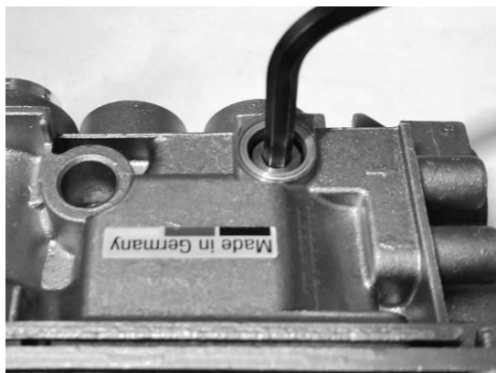
Figure 23 – Low Flow Orifice Removal
