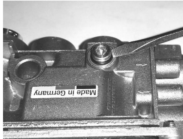
Figure 24 – Low Flow Orifice Removal – O-ring
