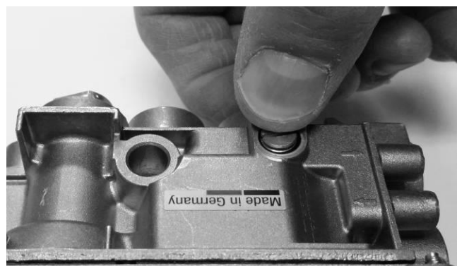
Figure 25 – NG Low Flow Screw Removal
