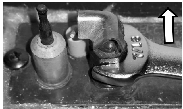
Figure 28 – Pilot in NG (Pilot Gate forward)
